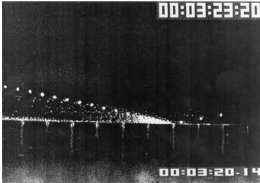
Figure 4. Collision of a saltating grain in the size range 0.2–0.25 mm with a bed of 0.05 mm grains.
